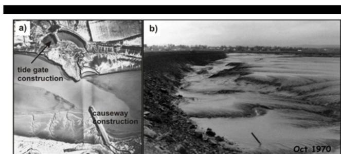
Figure 2: a) Rapid development of mudflat downstream of the Petitcodiac causeway in 1966, keeping pace with construction. Note dry land construction of tide gates; b) Rapid infilling of sediment adjacent to the Windsor causeway in Nov 1970.
