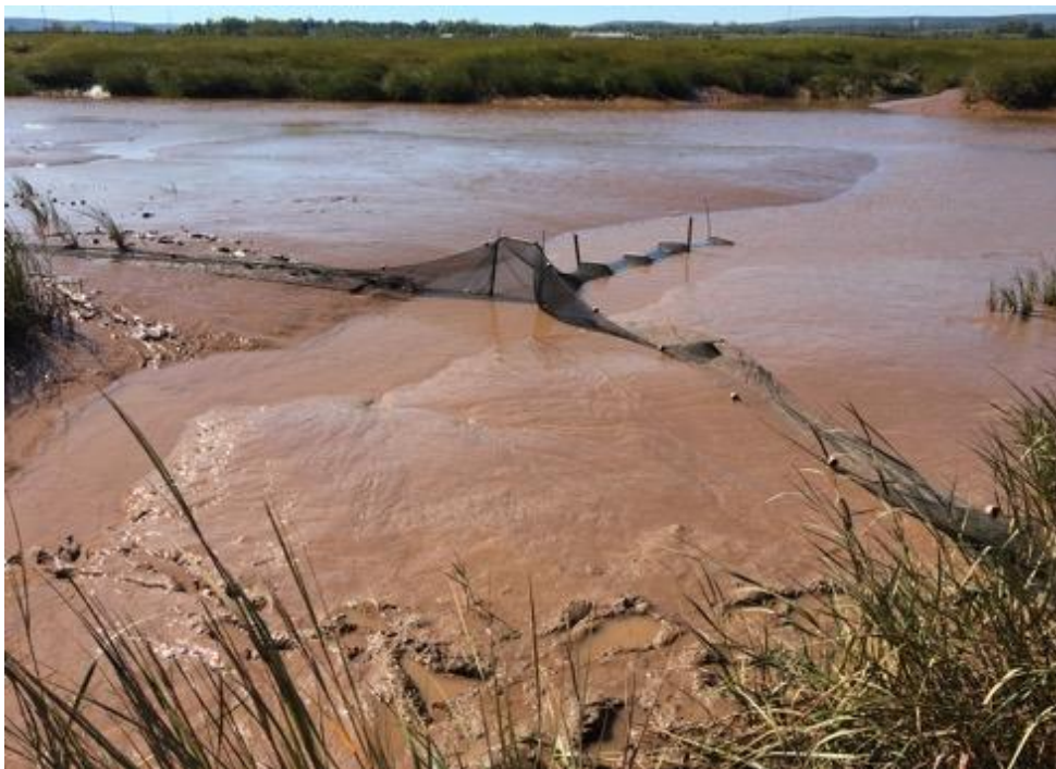
Figure 2 Fyke net deployed within secondary drainage channel on a falling tide on 27 September 2019.
