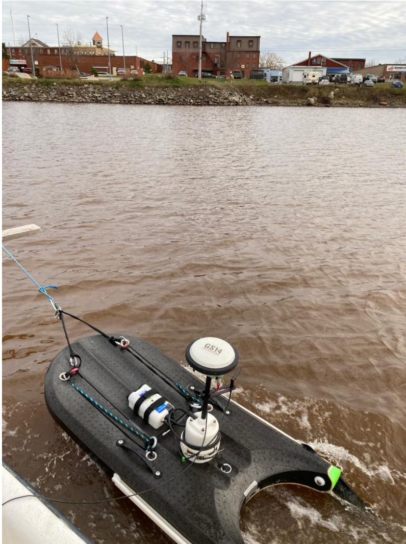
FIGURE 5: SONTEK M9 ON HYDROBOARD FOR BATHYMETRIC SURVEYING, DEC 11, 2020.
