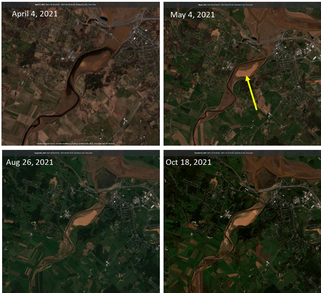
Figure 17: Copernicus Sentinel-2 satellite imagery (April – October 2021) illustrating sedimentation and evolution of intertidal bar and wetland vegetation after gates opened to allow for fish passage in March 2021. Arrow indicates position of sand bar and site of dust mitigation efforts.
