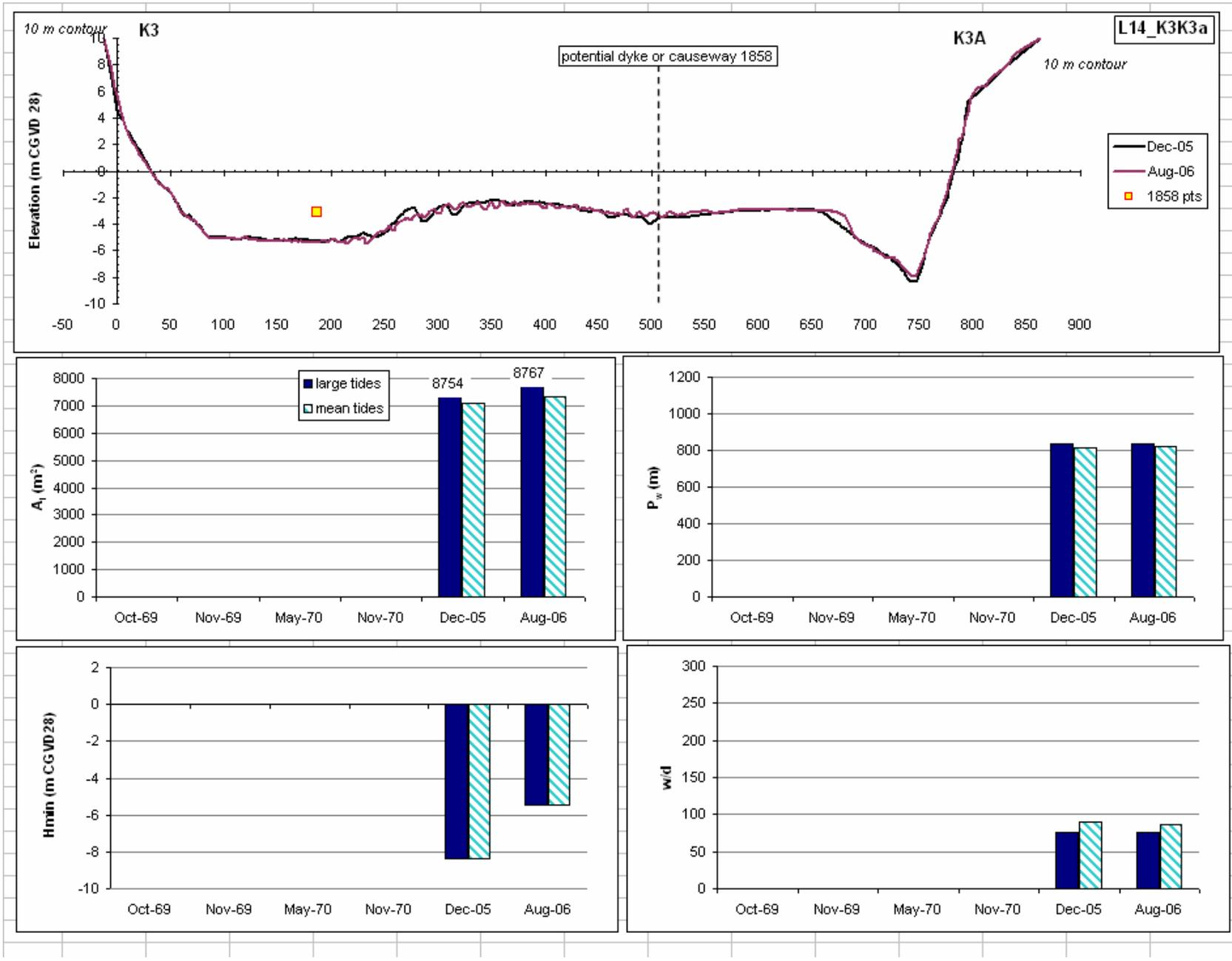
Figure 4.4c: Cross sectional profile for Line14\_DS\_K3K3A and associated hydraulic geometry parameters along the Kennetcook River. Vertical exaggeration on cross sectional profile = 42.5. Distance on cross sectional profile in metres. Note potential dyke or causeway that was visible on 1858 map. The position or existence of this dyke could not be verified and however since the thalweg was indicated as being along the opposite shore, it is possible.
