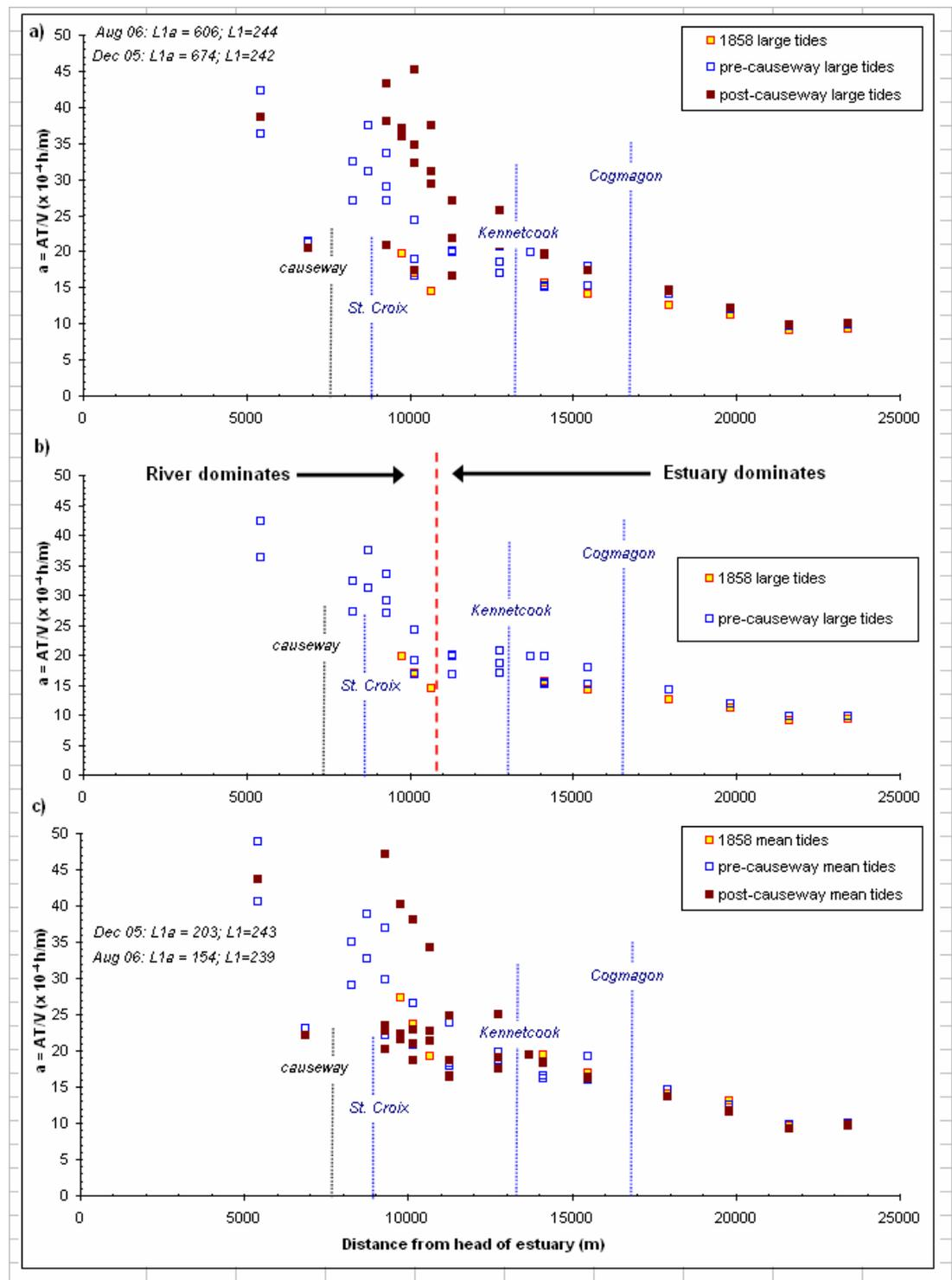
Figure 4.10: Variation in parameter 'a' ( $=AT/V$ ) (Bray et al., 1982) with distance from head of tide for a) large tides pre and post causeway; b) pre-causeway large and mean tides and c) mean tides pre and post causeway.  $A$  = intertidal cross sectional area,  $V$  = tidal prism above cross section and  $T$  = length of time during which there is tidal water in the channel
