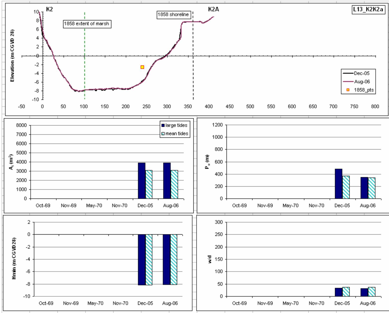
Figure 4.4b: Cross sectional profile for Line13\_DS\_K2K2A and associated hydraulic geometry parameters along the Kennetcook River. Vertical exaggeration on cross sectional profile = 42.5. Distance on cross sectional profile in metres.
