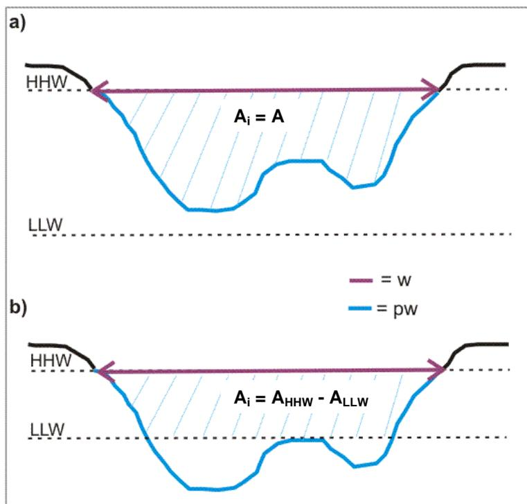
Figure 3.5 : a) Intertidal cross sectional area ( $A_i$ ) when LLW level falls below the lowest surveyed bed elevation; b) Intertidal cross sectional area measured as the difference between cross sectional areas calculated for HHW and LLW. The geodetic elevation of these tidal limits will vary depending on whether the calculations are being performed for large tides or average tides. Channel width (w) and wetted perimeter (pw) are also indicated.
