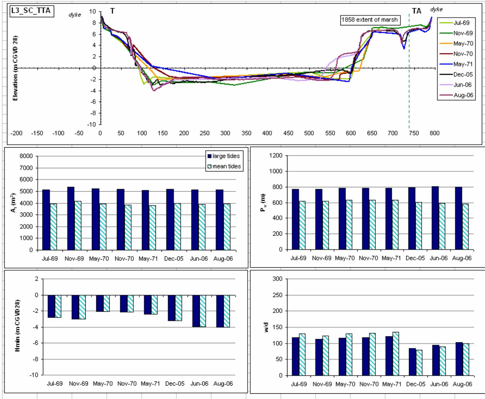
Figure 4.2c: Cross sectional profile for Line3\_SC\_TTA and associated hydraulic geometry parameters on the St. Croix River. Vertical exaggeration on cross sectional profiles = 50 X. Distance on cross sectional profile in metres. Refer to figure 4.1e for position of line.
