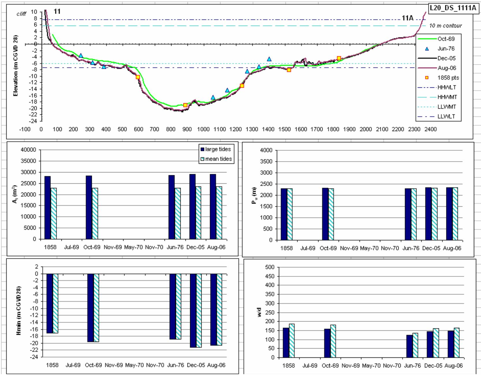
Figure 4.3w: Cross sectional profile for Line20\_DS\_1111A and associated hydraulic geometry parameters on the Avon River. Vertical exaggeration on cross sectional profiles = 73 X. Distance on cross sectional profile in metres.
