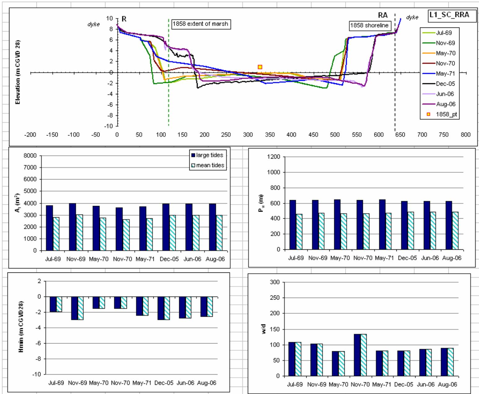
Figure 4.2a: Cross sectional profile for Line1\_SC\_RRA and associated hydraulic geometry parameters on the St. Croix River. Vertical exaggeration on cross sectional profiles = 50 X. Distance on cross sectional profile in metres. Refer to figure 4.1e for position of line.
