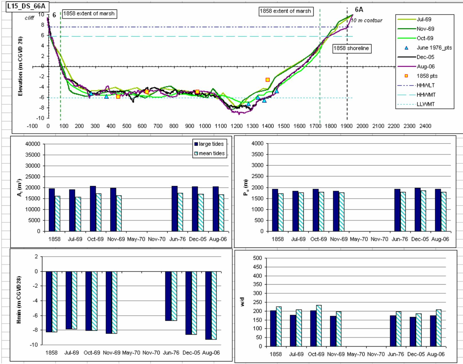
Figure 4.3p: Cross sectional profile for Line15\_DS\_66A and associated hydraulic geometry parameters on the Avon River. Vertical exaggeration on cross sectional profiles = 125 X. Note change in scale on y axis for cross sectional area and wetted perimeter. Distance on cross sectional profile in metres.
