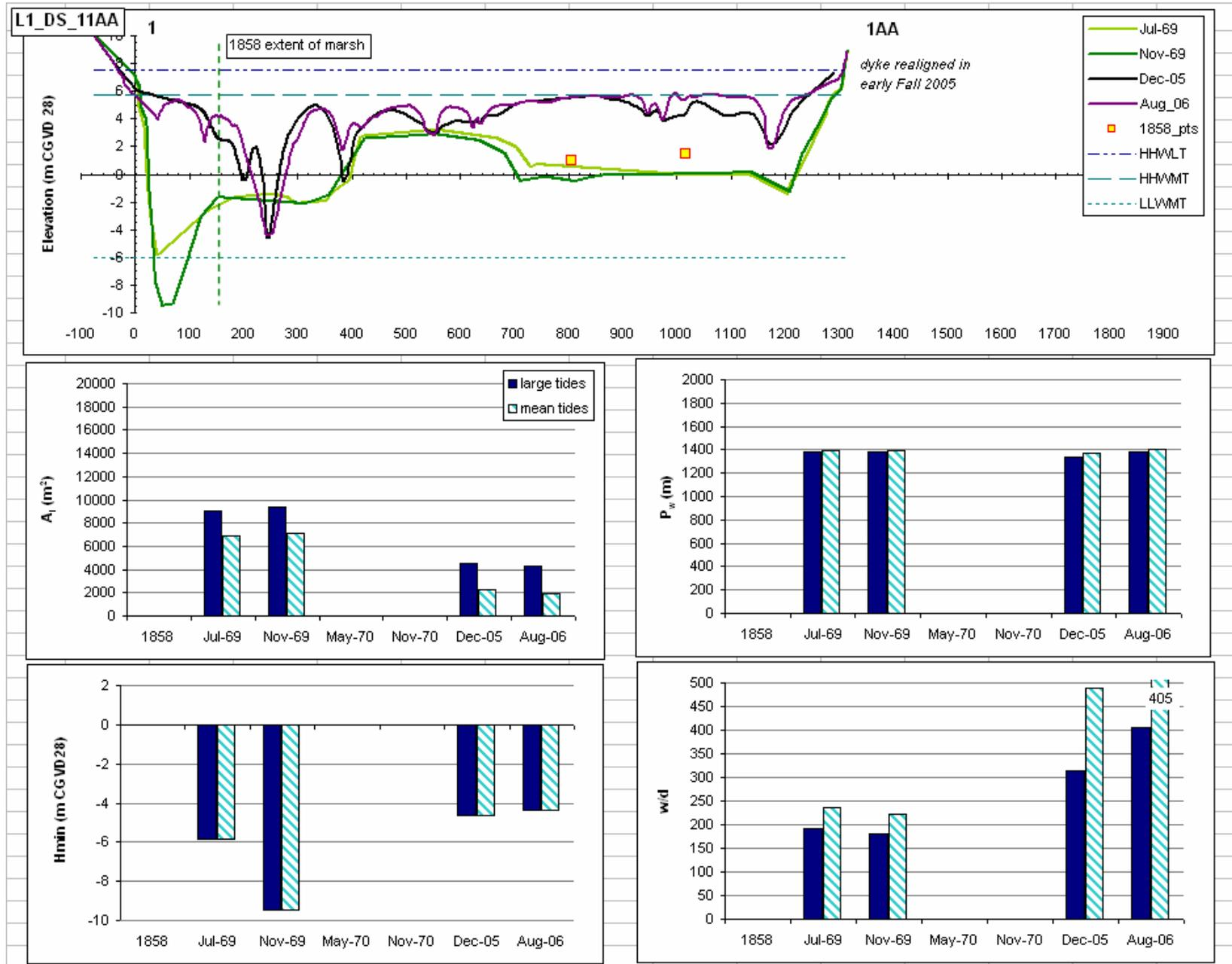
Figure 4.3e: Cross sectional profile for Line1\_DS\_11AA and associated hydraulic geometry parameters on the Avon River. Vertical exaggeration on cross sectional profiles = 100 X. Distance on cross sectional profile in metres.
