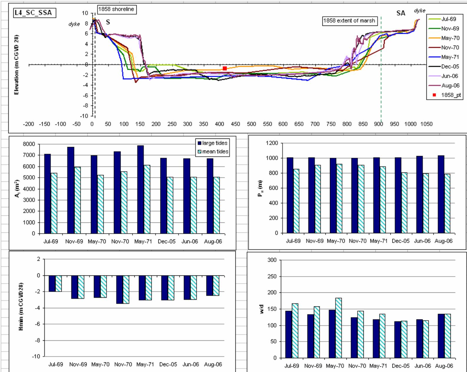
Figure 4.2d: Cross sectional profile for Line4\_SC\_SSA and associated hydraulic geometry parameters on the St. Croix River. Vertical exaggeration on cross sectional profiles = 50 X. Distance on cross sectional profile in metres. Refer to figure 4.1e for position of line.
