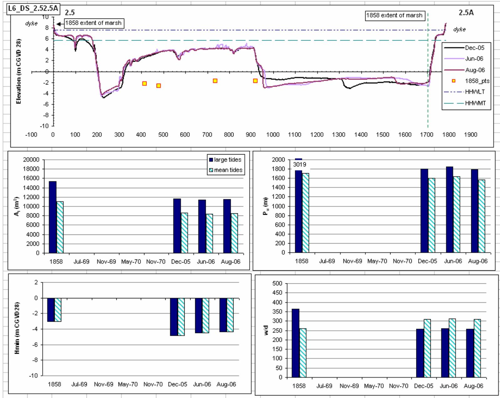
Figure 4.3h: Cross sectional profile for Line6\_DS\_2.52.5A and associated hydraulic geometry parameters on the Avon River. Vertical exaggeration on cross sectional profiles = 100 X. Distance on cross sectional profile in metres.
