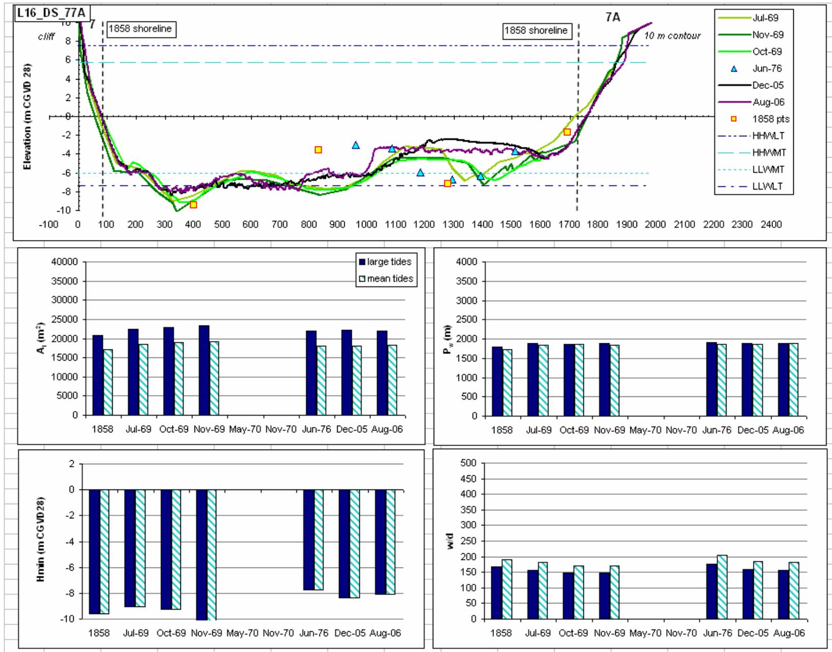
Figure 4.3q: Cross sectional profile for Line16\_DS\_77A and associated hydraulic geometry parameters on the Avon River. Vertical exaggeration on cross sectional profiles =125 X. Distance on cross sectional profile in metres.
