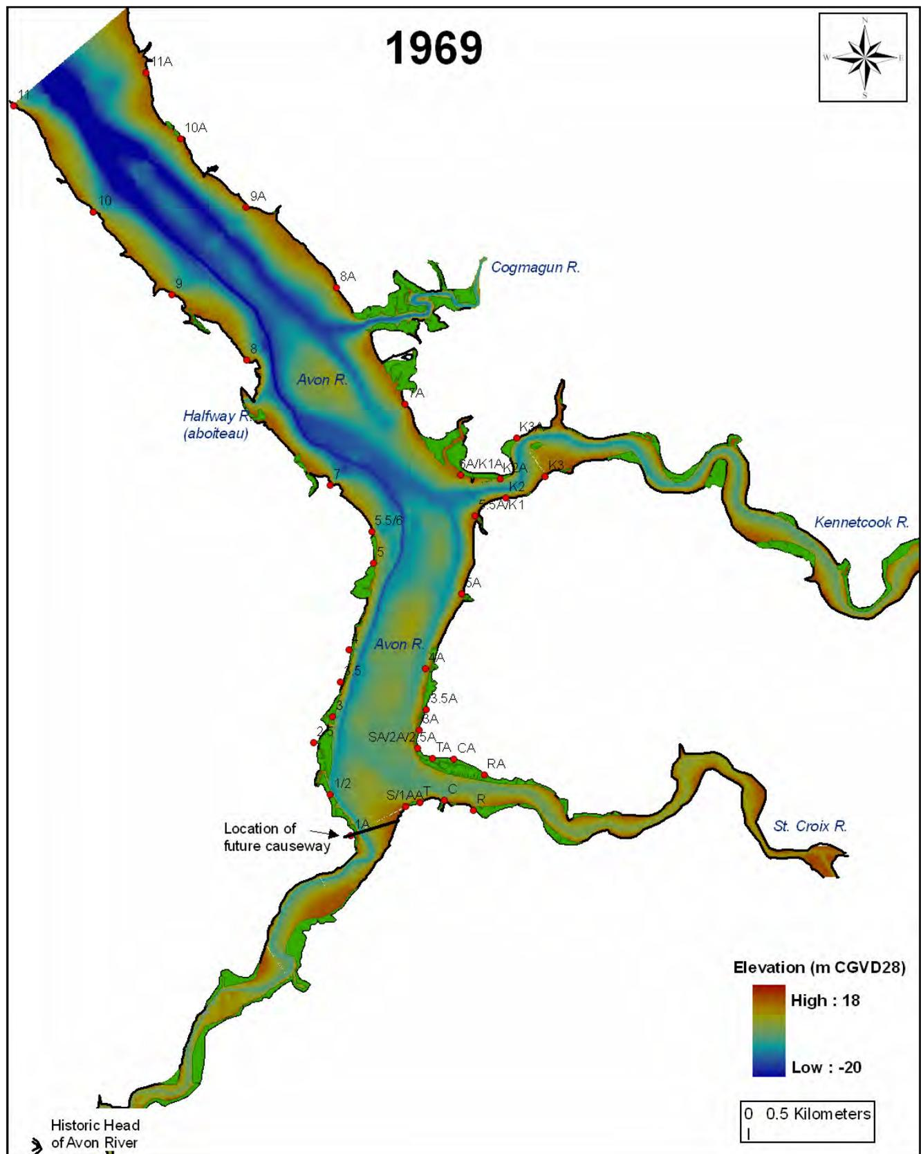
Figure 4.11b): Digital elevation model generated for 1969 for full tidal prism. Marsh areas for 1964 are in green and survey posts are provided for reference. Salt marsh in green. Dyked marshes excluded.
