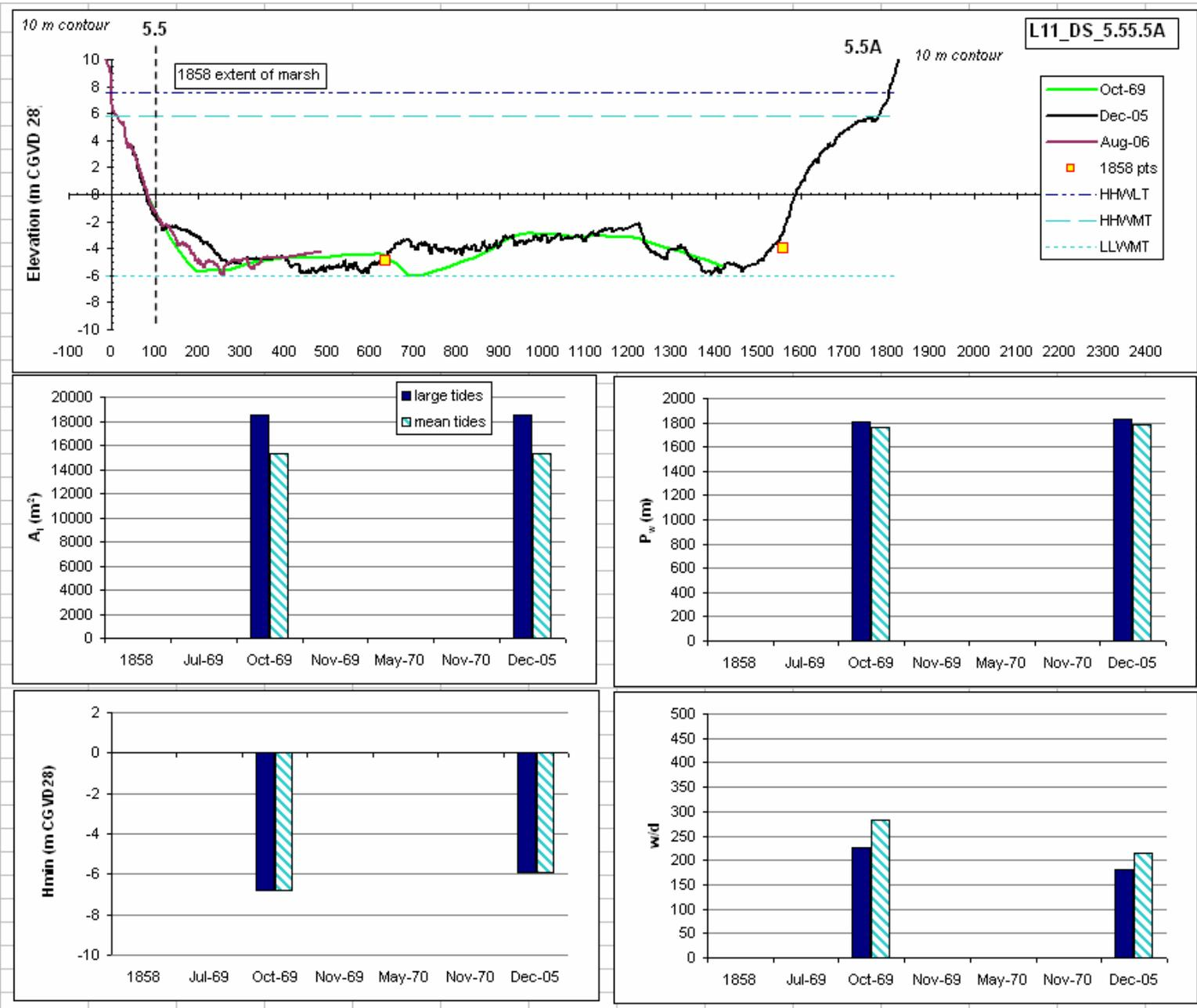
Figure 4.30: Cross sectional profile for Line11\_DS\_5.55.5A and associated hydraulic geometry parameters on the Avon River. Note change in vertical exaggeration on cross sectional profiles to 125 X. Distance on cross sectional profile in metres.
