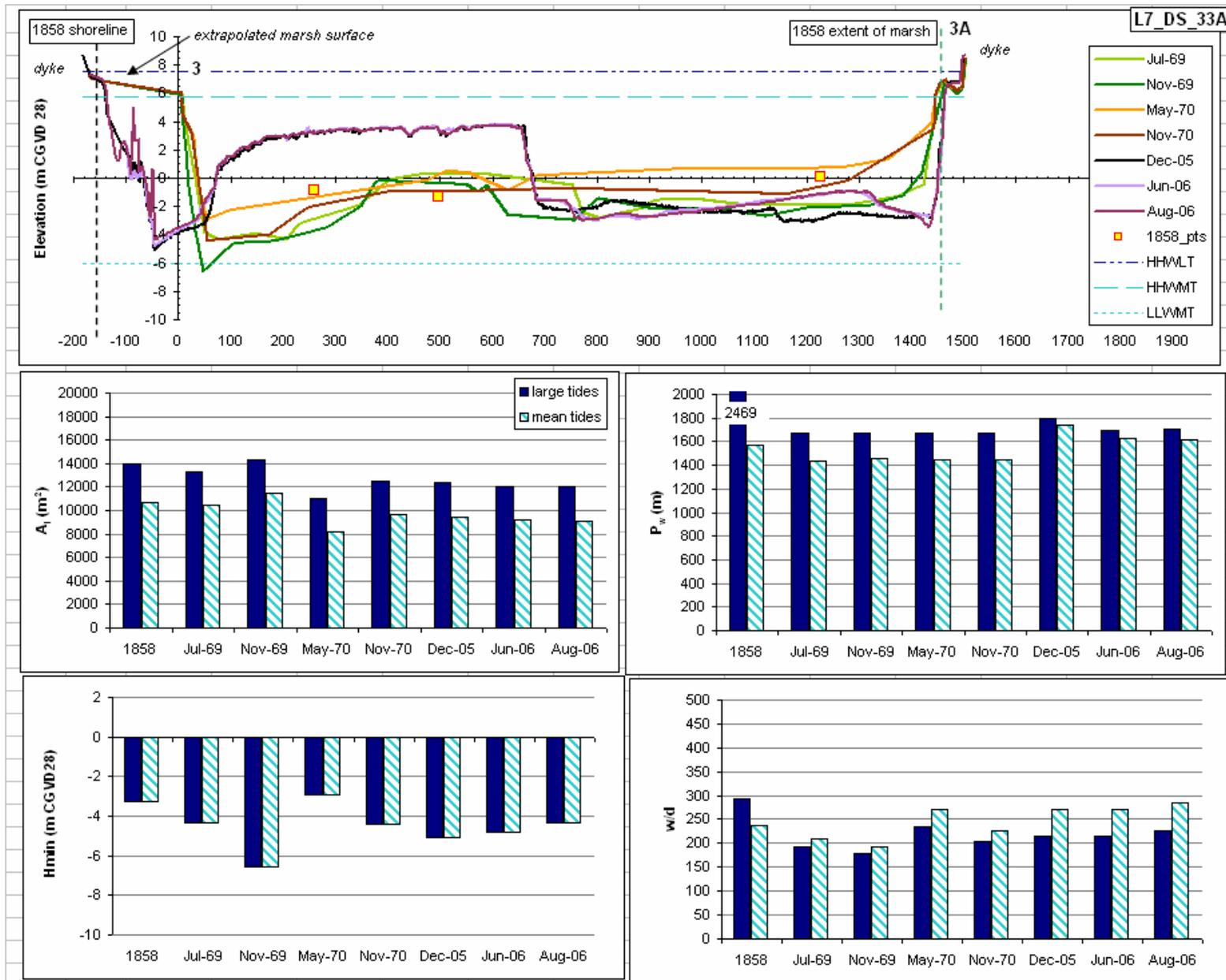
Figure 4.3i: Cross sectional profile for Line7\_DS\_33A and associated hydraulic geometry parameters on the Avon River. Vertical exaggeration on cross sectional profiles = 100 X. Distance on cross sectional profile in metres.
