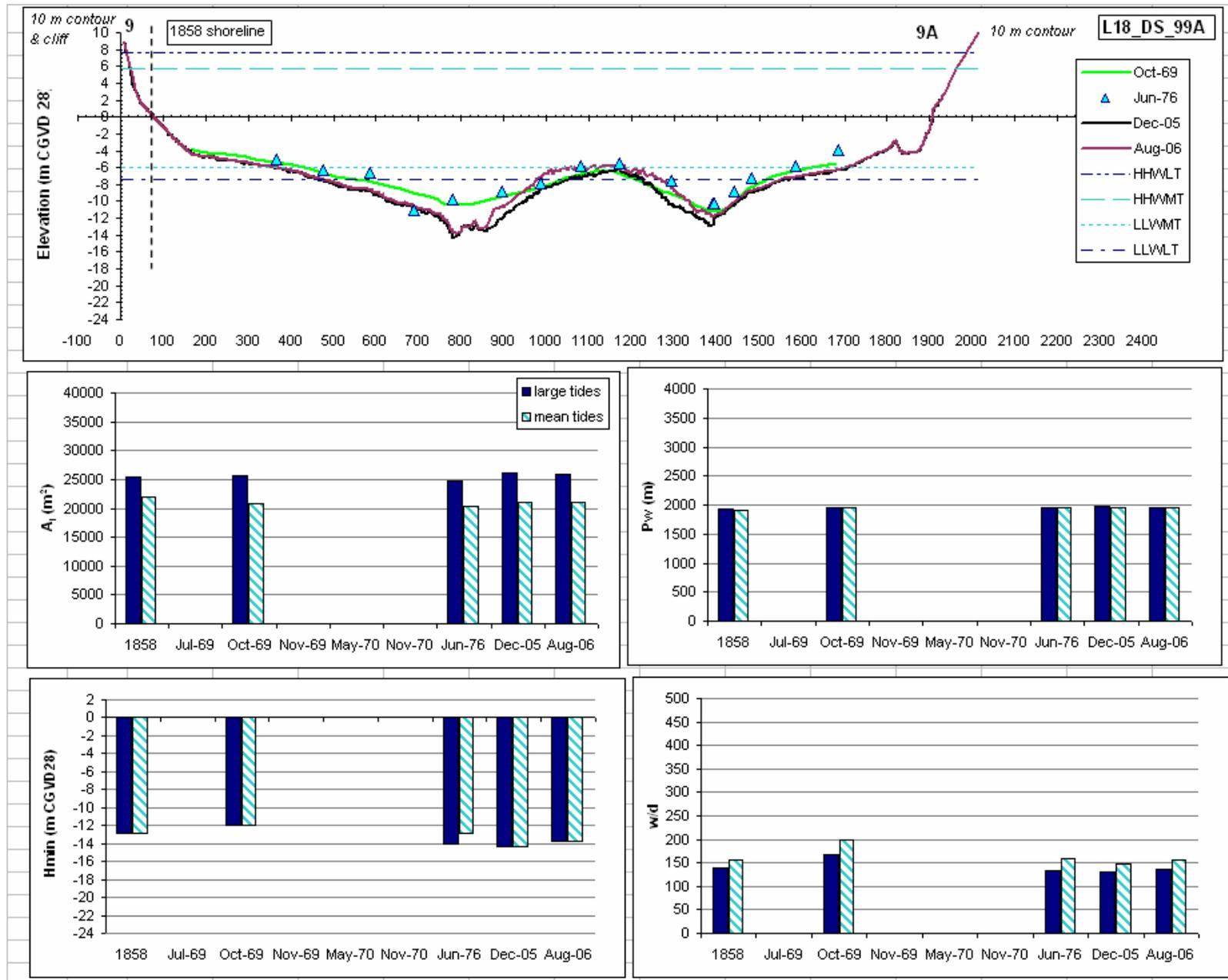
Figure 4.3t: Cross sectional profile for Line18\_DS\_99A and associated hydraulic geometry parameters on the Avon River. Vertical exaggeration on cross sectional profiles = 73 X. Note change in scale for minimum bed elevation. Distance on cross sectional profile in metres.
