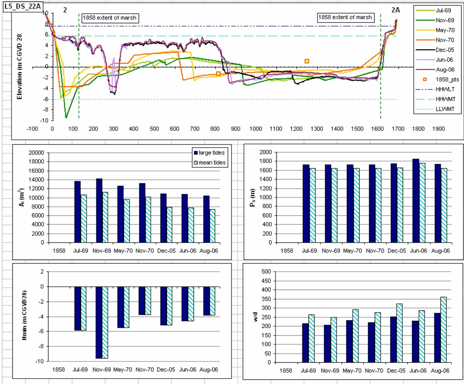
Figure 4.3f: Cross sectional profile for Line5\_DS\_22A and associated hydraulic geometry parameters on the Avon River. Vertical exaggaration on cross sectional profiles = 100 X. Distance on cross sectional profile in metres.
