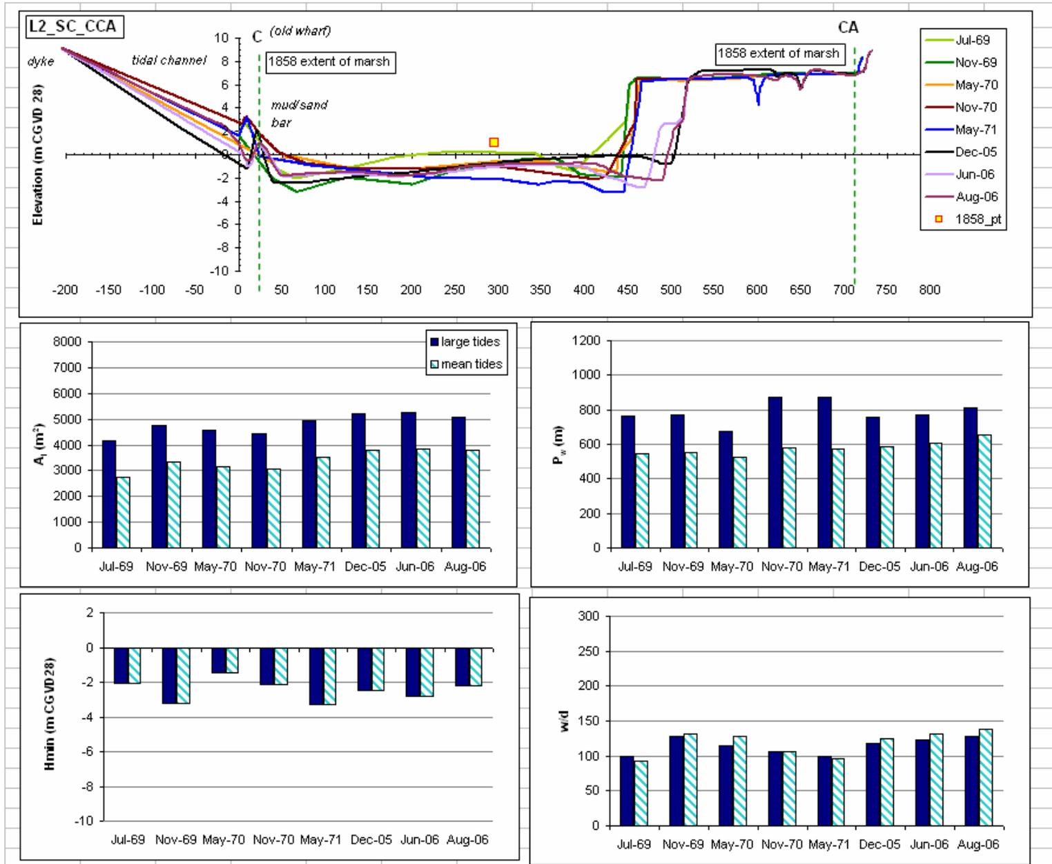
Figure 4.2b: Cross sectional profile for Line2\_SC\_C and associated hydraulic geometry parameters on the St. Croix River. Vertical exaggeration on cross sectional profiles = 50 X. Distance on cross sectional profile in metres. Prism and cross sectional area calculations are to be interpreted with some caution due to significant extrapolation on southern bank due to low elevation at the start of the survey and position of line within a tidal creek. Refer to Figure 4.1e for position of line.
