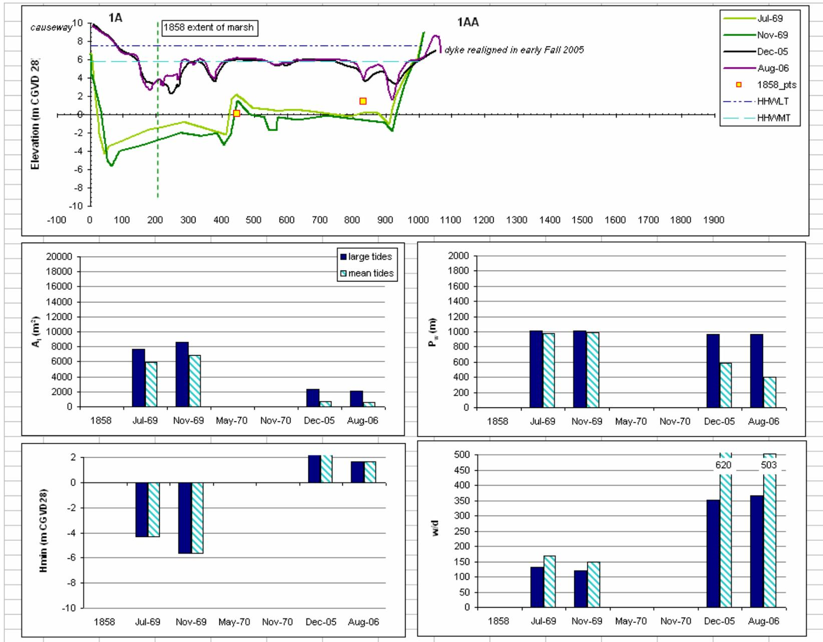
Figure 4.3d: Cross sectional profile for Line 1\_DS\_1A1AA and associated hydraulic geometry parameters on the Avon River. Note change in vertical exaggeration on cross sectional profiles to 100 X. Distance on cross sectional profile in metres.
