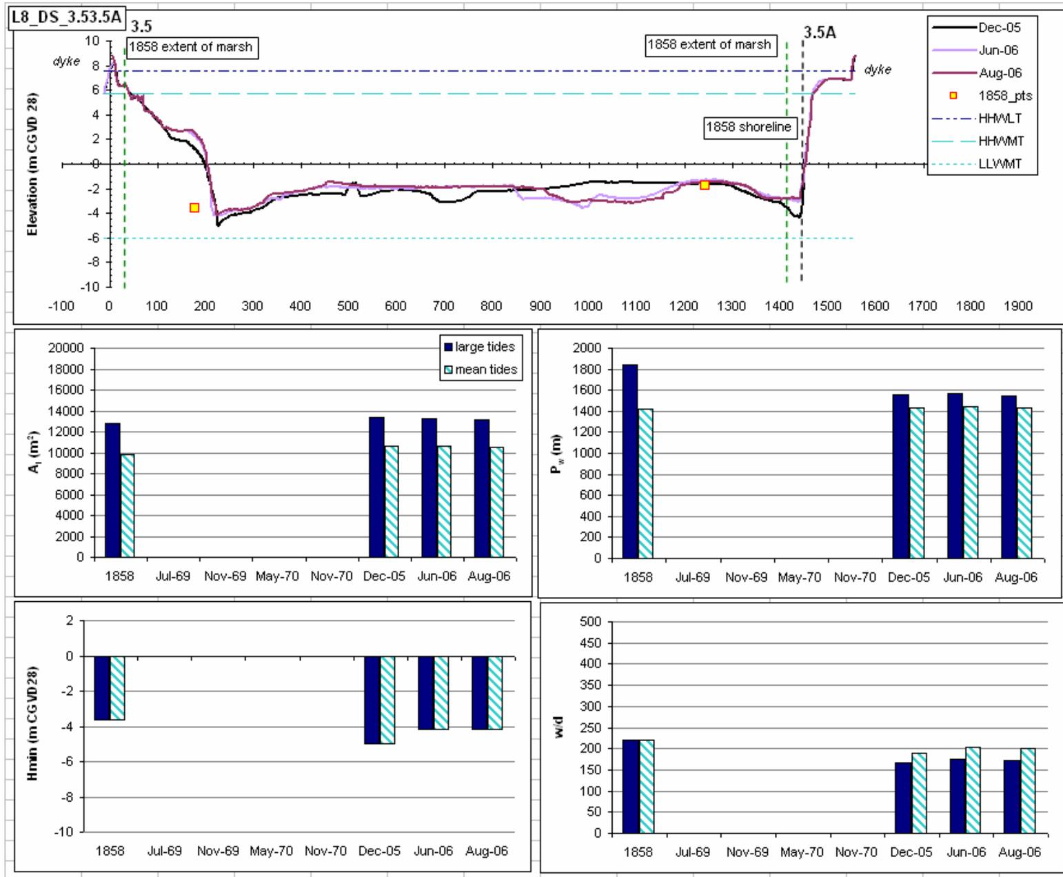
Figure 4.3j: Cross sectional profile for Line8\_DS\_3.53.5A and associated hydraulic geometry parameters on the Avon River. Vertical exaggeration on cross sectional profiles = 100 X. Distance on cross sectional profile in metres.
