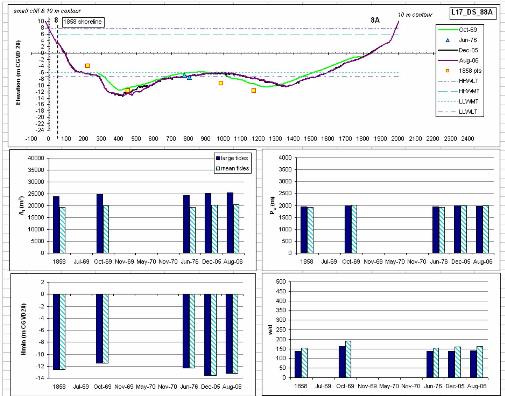
Figure 4.3s: Cross sectional profile for Line17\_DS\_88A and associated hydraulic geometry parameters on the Avon River. Note change in vertical exaggeration on cross sectional profiles to 73 X. Distance on cross sectional profile in metres.
