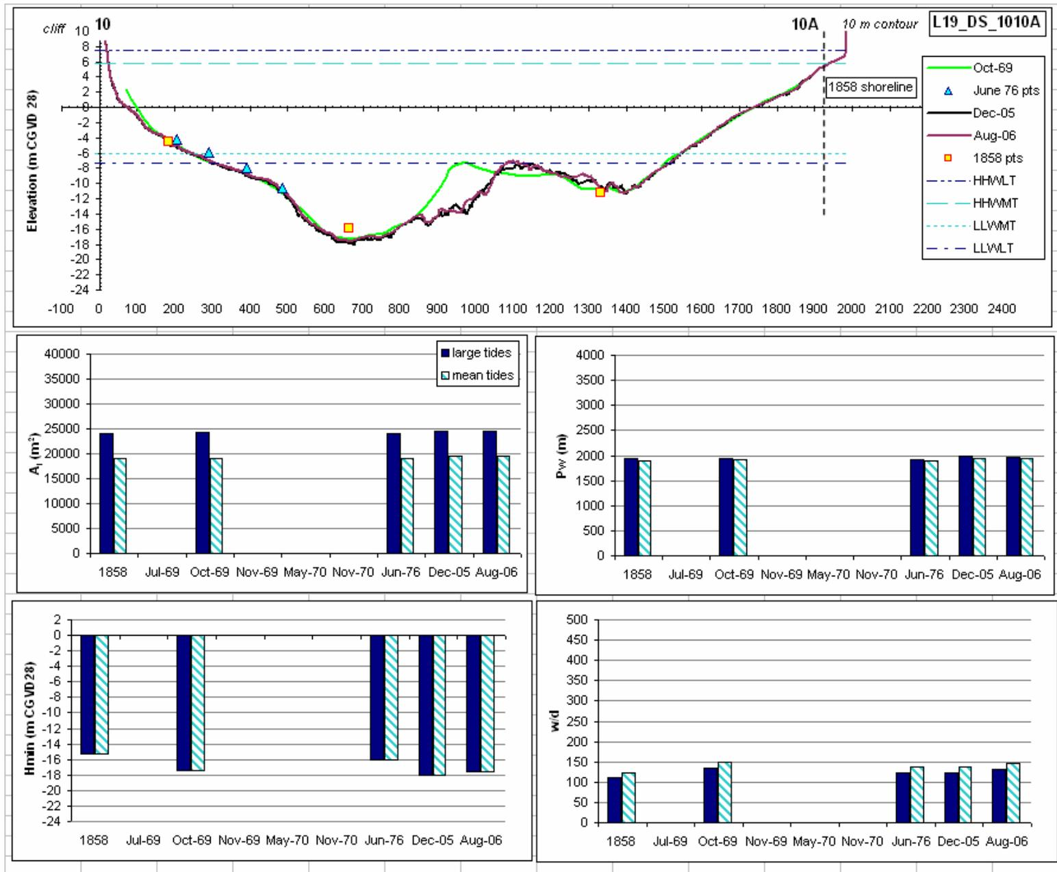
Figure 4.3v: Cross sectional profile for Line19\_DS\_1010A and associated hydraulic geometry parameters on the Avon River. Vertical exaggeration on cross sectional profiles = 73 X. Note change in scale for minimum bed elevation. Distance on cross sectional profile in metres.
