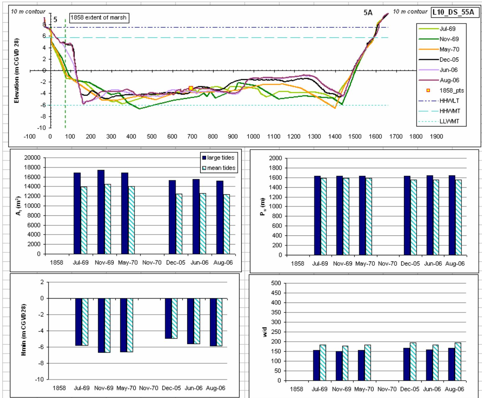
Figure 4.3m: Cross sectional profile for Line10\_DS\_55A and associated hydraulic geometry parameters on the Avon River. Vertical exaggeration on cross sectional profiles = 100 X. Distance on cross sectional profile in metres.
