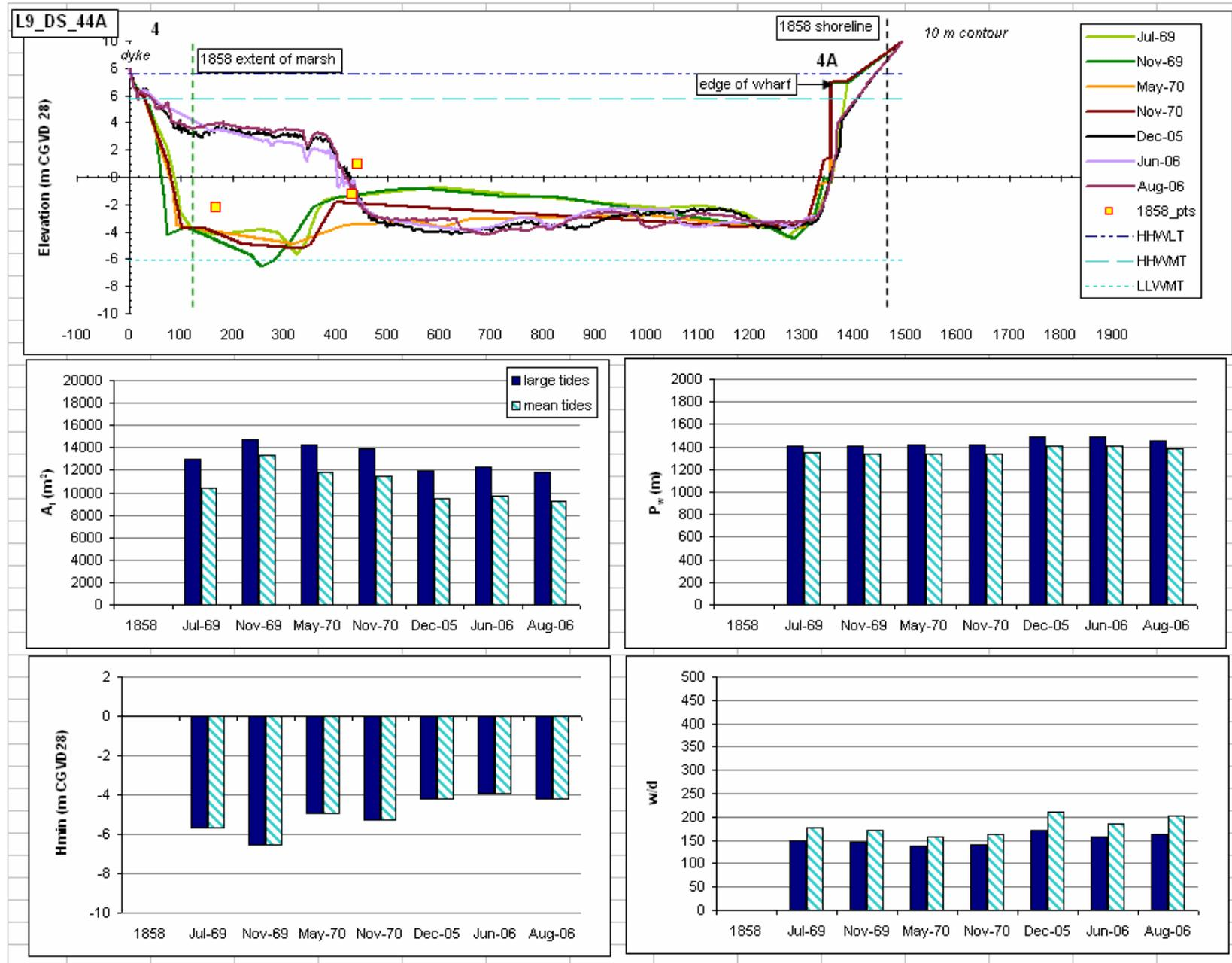
Figure 4.31: Cross sectional profile for Line9\_DS\_44A and associated hydraulic geometry parameters on the Avon River. Vertical exaggeration on cross sectional profiles = 100 X. Distance on cross sectional profile in metres.
