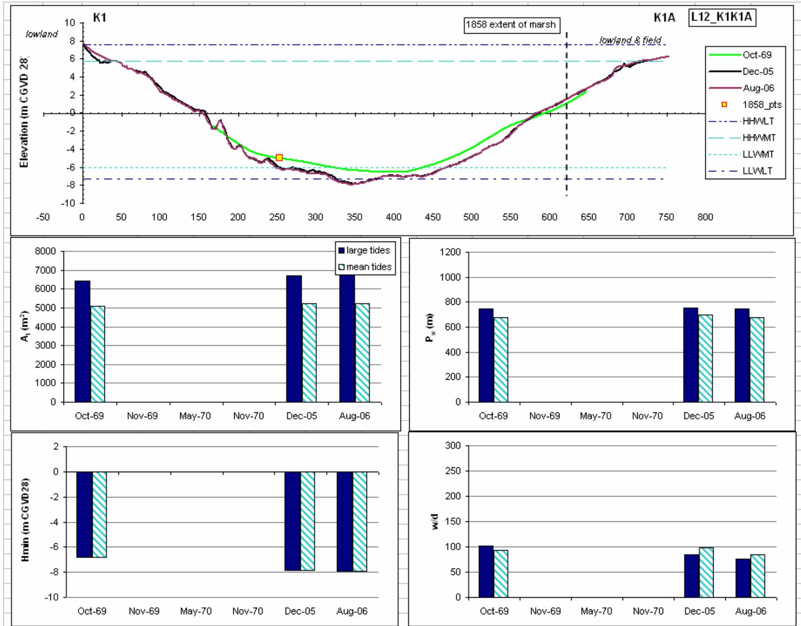
Figure 4.4a: Cross sectional profile for Line12\_DS\_K1K1A and associated hydraulic geometry parameters along the Kennetcook River. Vertical exaggeration on cross sectional profile = 42.5. Distance on cross sectional profile in metres. The section of the profile near K1A could not be extended further due to the extensive lowland area adjacent to it.
