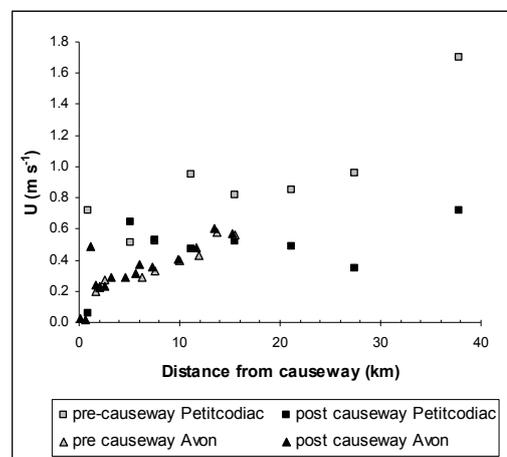
Figure 4. Variation in critical tidal velocity pre and post construction at HHWLT.
