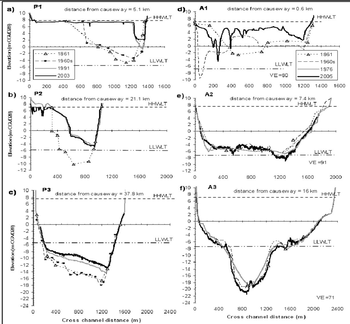
Figure 3. Variation in tidal channel cross sections on the Petitcodiac (a-c) and Avon (d-f) rivers since the 1860s. Elevations are in meters relative to the Canadian Geodetic Vertical Datum CGVD28. HHWLT=higher high water large tides, LLWLT=lower low water large tides.
